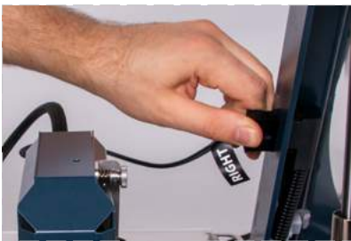
Connect the LEFT cable to the LEFT frame socket and RIGHT cable to the RIGHT frame socket.
