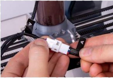
Connect the 'A' cable to the A cable from X-carriage.
