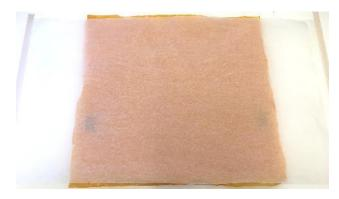
Use an iron which is turned up to the highest temperature to laminate the plastic sheets together. Begin in the centre and use a circular or zigzag motion to cover the whole area. Ensure you apply pressure and spend enough time across the whole area to fully fuse the layers together.
