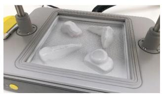
Carefully cut away the excess around the car designs with a pair of scissors.
