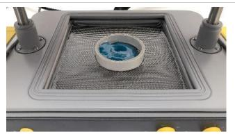
Allow the plastic to cool and remove the whole thing from the FormBox. Gently pull the models out.
