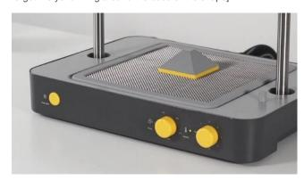
When the plastic is ready you will see ripples at the edges of the sheet and a droop in the middle. Form the template with the Mayku Cast Sheet.
