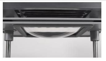
Allow the plastic to cool and remove the whole thing from the FormBox. Gently remove the models.
